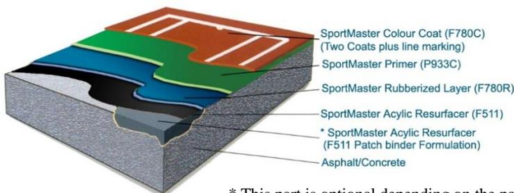
\* This part is optional depending on the pavement condition and profile of surface.
