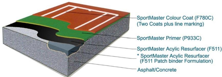
\* This part is optional depending on the pavement condition and profile of surface.
